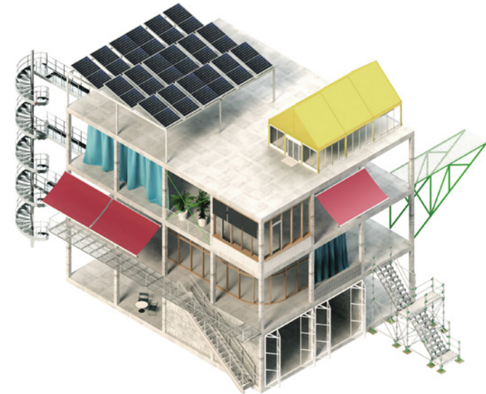
Conceptual representation illustrating the distinction between a load-bearing structure ( Hardware ) and flexible architectural solutions ( Software ) that enable required functions and create necessary environmental conditions, Artem Kitaev
