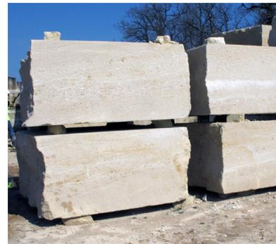
Fig 3 - The blocks extracted from the quarry are waiting to be squared, and to become architectural elements ready to be laid.
