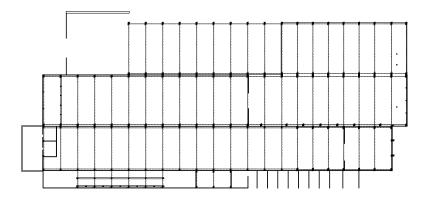
Primary Structure 2021, ElBeton prefab factory, Aalter. Plan by Tycho Maes and Alexandre Moens. In this drawing the system of different sheds built alongside each other is shown.
