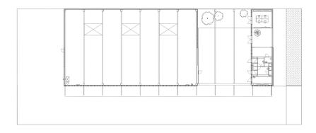
G1812 Industrial building, Gent (BE), 2021, GAFPA. Plan to illustrate the placement of the building in the right corner of the plot. Production hall and offices in one space seperated by a canopy.
