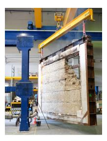
Fig. 22 - Fire resistance test.
