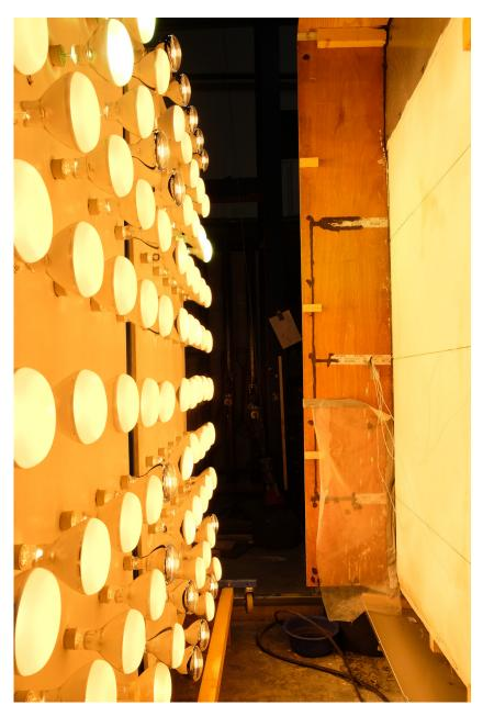
Fig. 24 - The photo shows the drying bench which generates a temperature of  $80^{\circ}\text{C}$  for the drying cycle.
