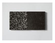
Figure 1b: The Shanxi Black Granite originates from China, and was provided and produced by Potier Stone in Maldegem (BE). The Recycled Polyurethane Foam was provided and produced by Stuntmarkt in Zwijndrecht (NL).
